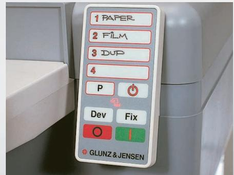
The detachable control panel contains all necessary operating indications, e.g. low-level, deviation of temperature and wait signal.
